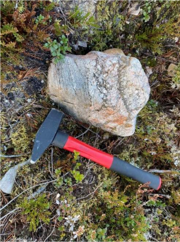
Figure 5. Tonalitic gneiss sample from moraine. Both neosome and leucosome (tonalitic) are visible.
